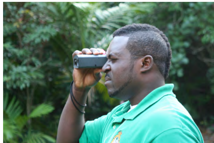
Figure 16: Bahamas National Trust Park Warden, Apollo Butler He uses a rangefinder to measure the distance to the birds he is counting. Photo by Geoff Welch
