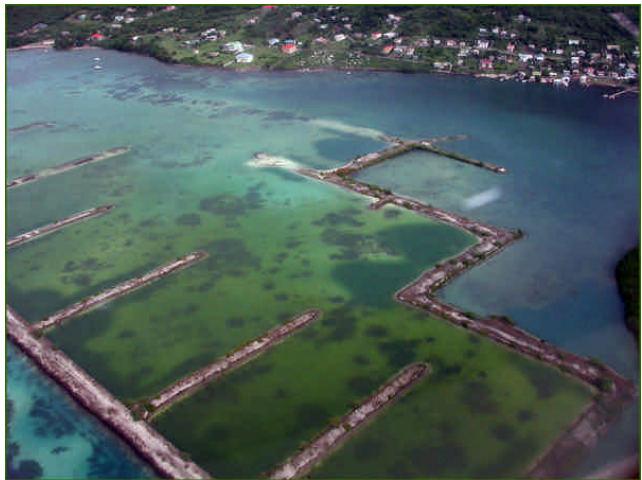
Aerial photo of Ashton Lagoon causeway and marina berths showing stagnant eutrophic water in the lagoon (2004)
