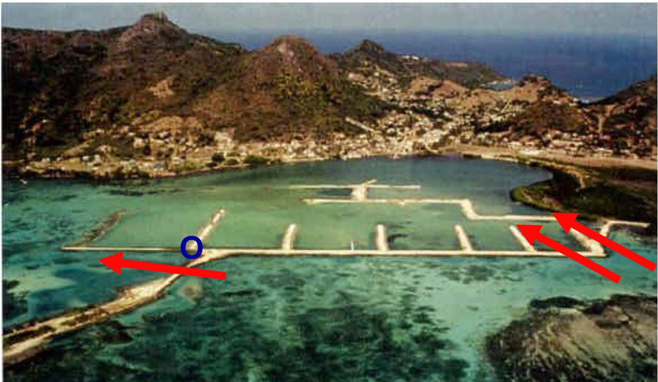
Figure 2. Red arrows show locations discussed in text where the causeway should be opened to restore flow. The tail end of Frigate Island is at lower left. The blue circle is the suggested location for the power supply for Biorock projects and a future office and visitor centre. This location would allow power to be supplied for Biorock projects on both sides in much of the central Lagoon. Photograph by Stephen and Purnima Price.
